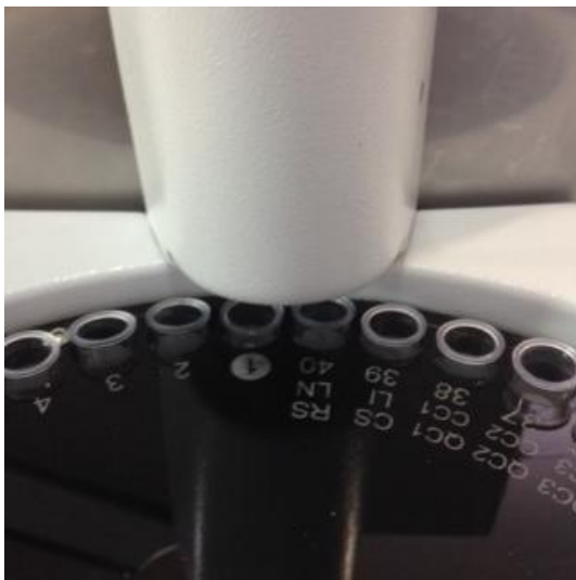
Needle not correctly centered.
