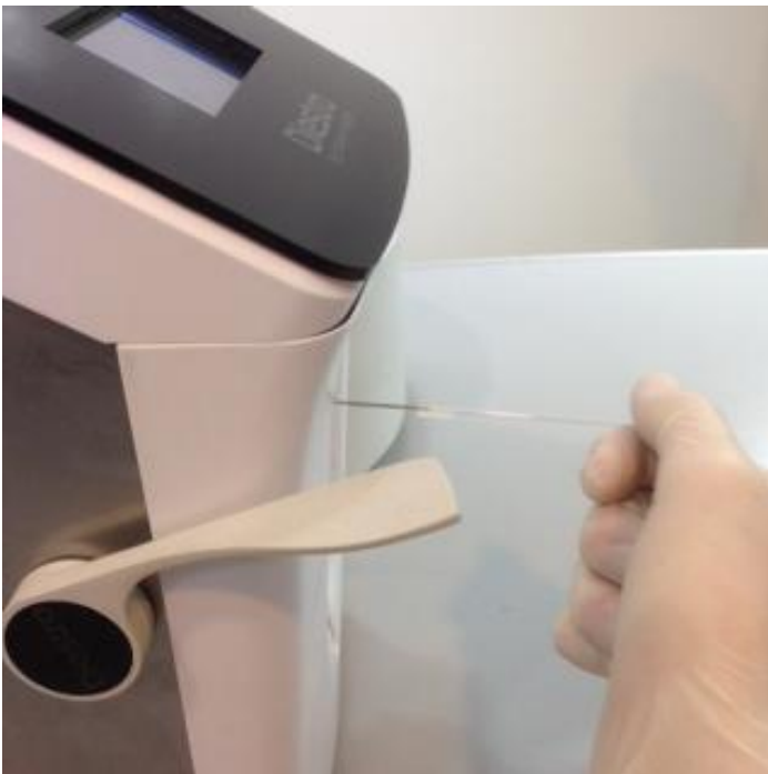
Load from a capillary
