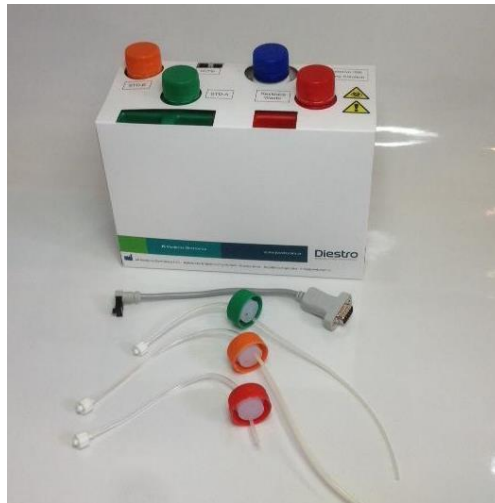
View of the Pack and its connection pipes
